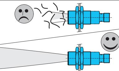
The transducer surface as well as the field of the detection beam must be kept free mandatorily. You need to pay attention on having no disturbing objects between the sensor and the target object within the detection beam.
