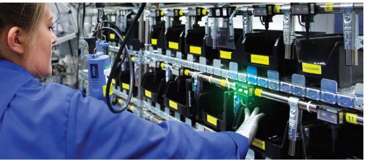
Lights or doors guide the operator to the correct box
