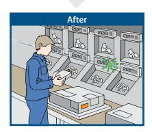
In a typical application, where personnel are required to pick a number of different parts or products from bins in sequence, the chances of the worker correctly picking the parts with 100 % reliability every time are small. At the very least, a significant proportion of the production time will be taken up by looking for the right part and ensuring that it is indeed
